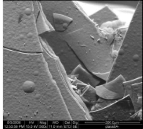
Fig. 4: A secondary electron image of a cross section through corroded crusts of the bottle (A00). The distinction between original glass, leached layer and surface crust cannot easily be made.
