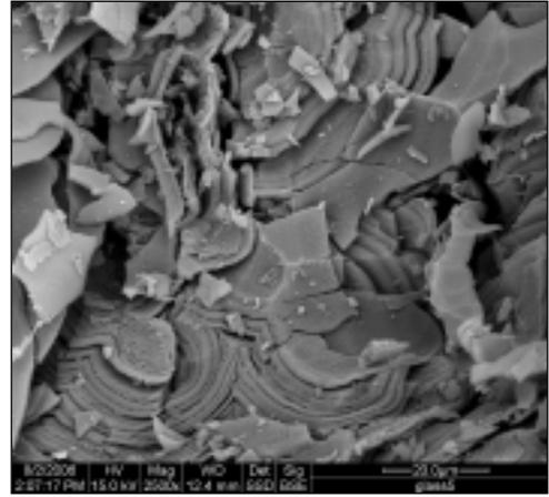
Fig. 2: A backscattered electron image of fragile crusts of glass bottle (A612) showing large areas of the weathering crusts be destroyed and rich in dissolution voids.
