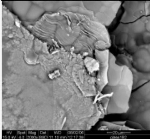
Fig. 1: A secondary electron image of a cross section through corroded crusts from the glass plate (A301) showing deterioration proceeding from the surface to the interior.
