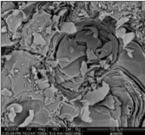
Fig. 3: A backscattered electron image of corroded crusts of glass bottle (A613) showing the weathered layers be destroyed, and losses its glassy nature.
