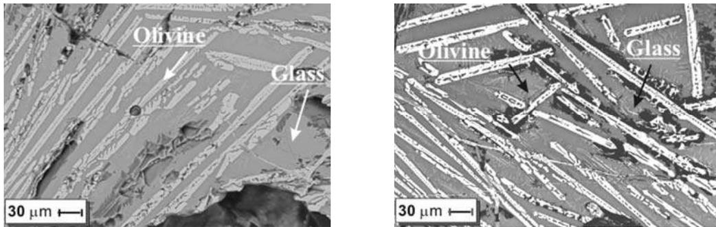
Fig. 5 SEM (BSE) images of iron slag. Fayalite elongated crystals are discernible in the vitreous groundmass.
