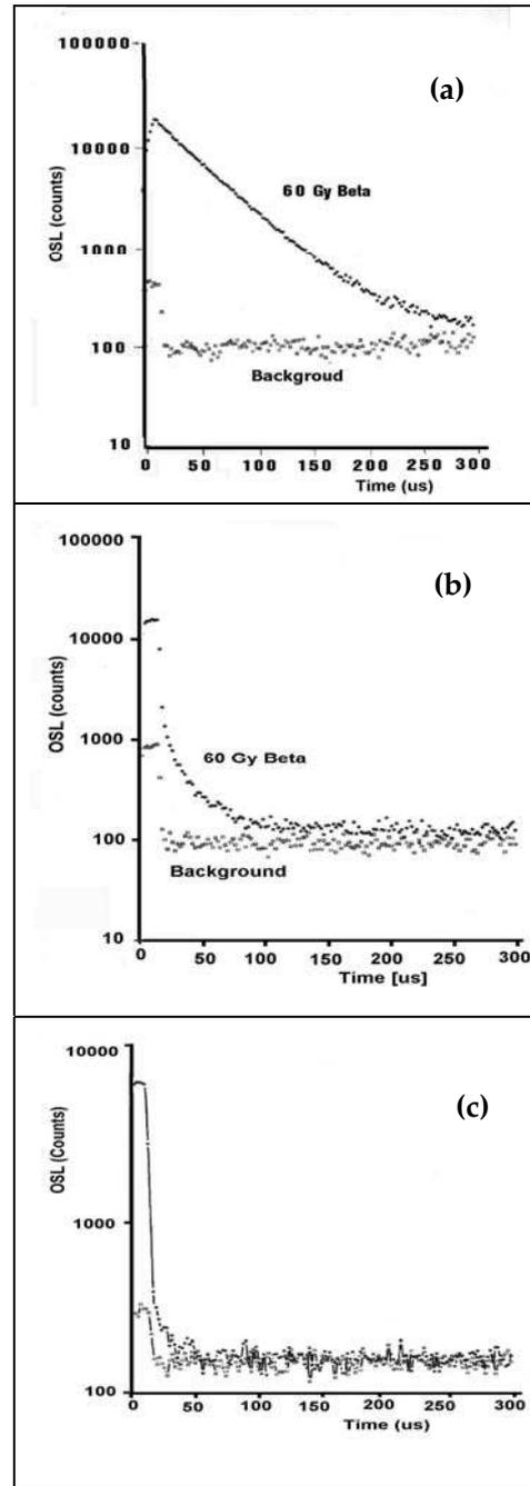
Fig.12 EGOS-7, granite. Stimulation by pulsed blue LED of, (a) daylight bleached quartz, with background and addition of 60 Gy, (b) daylight bleached orthoclase, with background and addition of 60 Gy, and (c) SOL bleached with background and addition of 40 Gy.
