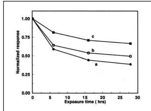
Fig.14 EGOS-7. The reduction of TL due to the solar bleaching is plotted in a normalized response for three different temperature regions, that is 280-350°C, 360-400°C and 410-450°C after 30 hrs the bleach approaches a plateau.
