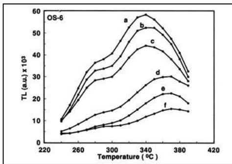
Fig.4 EGOS-6. Bleaching of TL after exposure to sunlight, a) geological TL, b) 2 hrs c) 8 hrs, d) 16 hrs, e) 24 hrs, f) 60 hrs.
