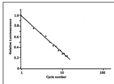
Fig.17f EGBAS, basalt. Decay curves for repeated preheat (300 sec at 220°C) and read (0.1 sec by blue LEDs) cycles, for material with SOL bleached for 6.5 hours, added 50 Gy dose.
