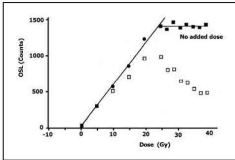
Fig.17b Single aliquot additive dose determination of ED. Exposure of EGBAS to 7 hours of SOL left no residual signal (ED=0.2±0.8 Gy).
