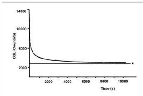
Fig.16b EGBAS, basalt. Bleaching by blue LEDs, for the whole 3 hours of measurement. The curve fitted to the data is the sum of 4 exponentials, with lifetimes  $1.1 \pm 0.1$ ,  $39 \pm 1$ ,  $438 \pm 18$  and  $4699 \pm 46$  sec.
