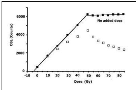
Fig.17c Single aliquot additive dose of EGBAS, by blue LEDs for ED determination, for the shorter preheating (ED=4±0.4 as the average of average of 3.8±0.4, 3.9±0.4, 4.4±0.5).
