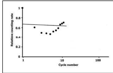
Fig.8 EGMKY after 3 hours SOL and 100 Gy, preheating for 300 sec at 220°C and 0.1 sec blue shine per cycle. It is interesting to note the competing mechanisms between bleaching and phototransfer taking place simultaneously; bleaching dominating at first, phototransfer dominating later.
