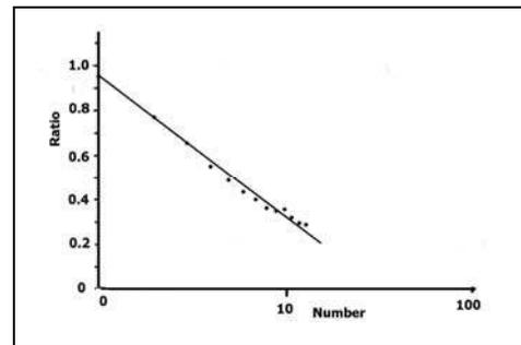
Fig.17e EGBAS, basalt. Decay curves for repeated preheat (60 sec at 220°C) and read (0.1 sec by blue LEDs) cycles, for material with the natural+50 Gy dose.
