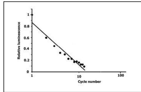
Fig.19a EGBAS, basalt. Decay OSL after exposure to SOL for 5.5 hrs, and take readings of 1 sec by IR with preheating at each cycle of 300 sec at  $220^\circ\text{C}$ . The fitting follows exponential law.
