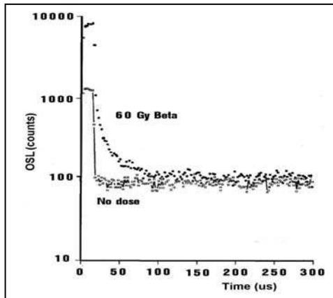
Fig.11 EGOS-7, granite. Stimulation by Pulsed blue LED, of daylight bleached microcline with no dose and with addition of 60 Gy,
