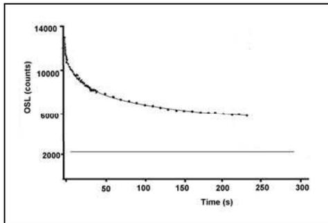
Fig.16a EGBAS, basalt. Bleaching by blue LEDs, for the first 250 sec. The straight line is the background, and the curve fit to the data is the sum of three exponentials.
