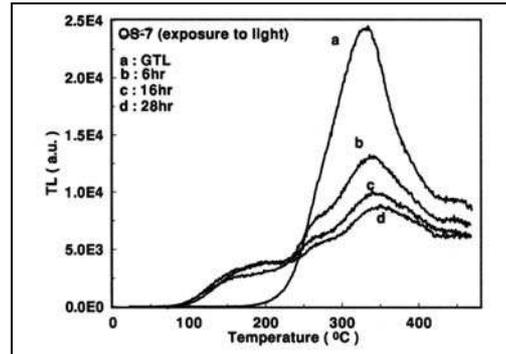
Fig.13 EGOS-7. Bleaching of TL after exposure to sunlight for a) geological TL, no exposure, b) 6 hrs, c) 16 hrs and d) 28 hrs.
