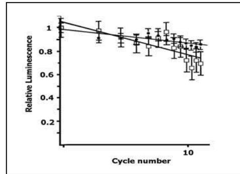
Fig.17d EGBAS, basalt. Decay curves for repeated preheat (60 sec at 220°C) and read (0.1 sec by blue LEDs) cycles, for material with the natural dose, compared with exposure to light only (with lower slope).
