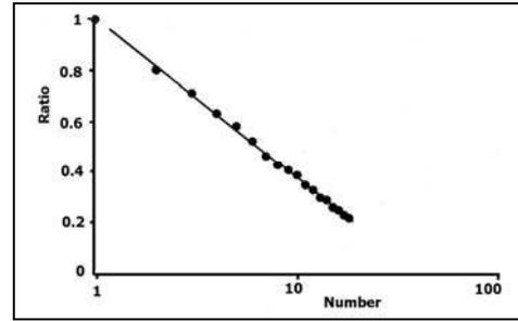
Fig. 10 EGOS-7 added 20 Gy and repeated preheat and read cycles by blue LEDs. The ratio is characteristic of feldspar,  $1 - a \ln(n)$ .
