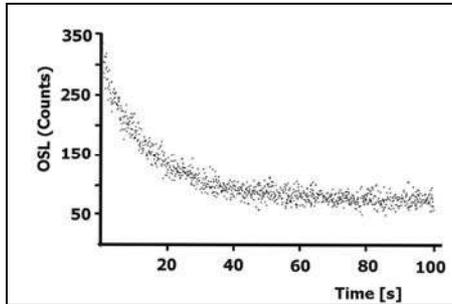
Fig.1 Bleaching of EGOS-6 by blue LEDs (sample irradiated with 20 Gy beta source, following the preheat/read sequence of fig.2).
