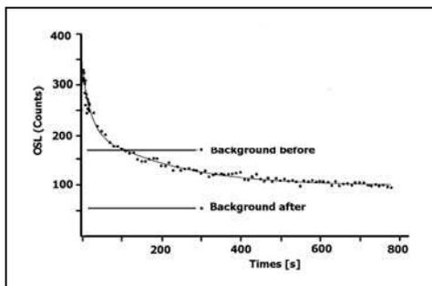
Fig.18 EGBAS, basalt. Natural bleaching by IR LEDs. Note the background before and after the reading. The curve is the sum of two exponentials (lifetimes  $20 \pm 2$  and  $208 \pm 22$  sec)
