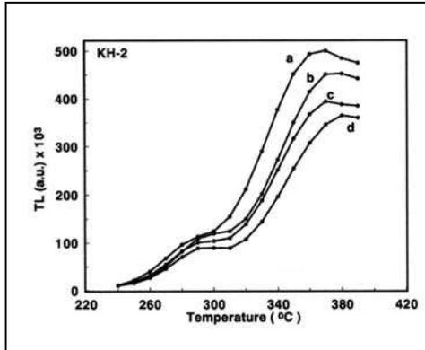
Fig.21 TL glow curves of EGKH, limestone. Solar bleaching as a function of exposure time, a) geological TL, b) 16 hrs, c) 25 hrs, d) 50 hrs.
