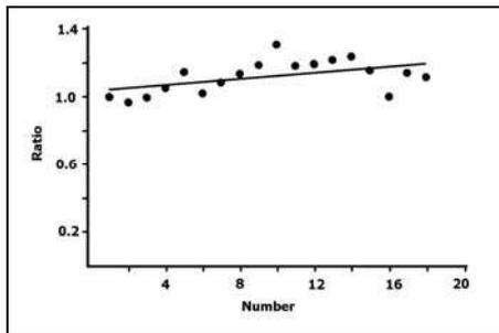
Fig.2 After a 20 Gy irradiation with a beta source, following 18 repeated preheatings and readings with 0.1 sec of blue LEDs, the signal was unusually constant.
