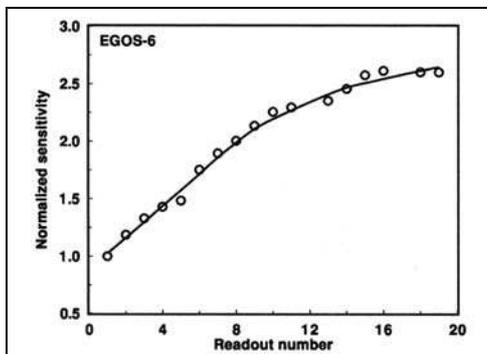
Fig.5 EGOS-6. TL sensitivity changes as a function of readout cycles (to 400°C). The increase is rapid (more than a factor of 2) for the 10 cycles, becoming lower towards the 20<sup>th</sup> cycle (by a factor of 2.7)
