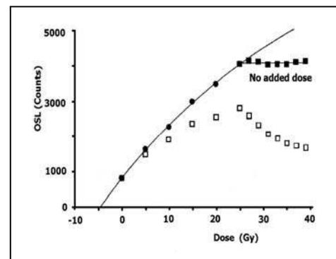
Fig.17a EGBAS, basalt. Following the relationship for relative luminescence of  $1 - \ln(n)$ , for higher preheating time 300 s at  $220^\circ\text{C}$  the single aliquot additive dose measurements gave  $\text{ED} = 4.7 \pm 0.5$  Gy.
