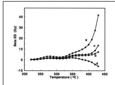
Fig.22 ITH-4, Determination of longer plateau. The best plateau is obtained for bleaching of 1-2 days in the temperature region 350-420°C. Curves correspond to a) no bleaching, b) 20 hrs bleaching, c) 2 days, and d) 6 hrs bleaching.
