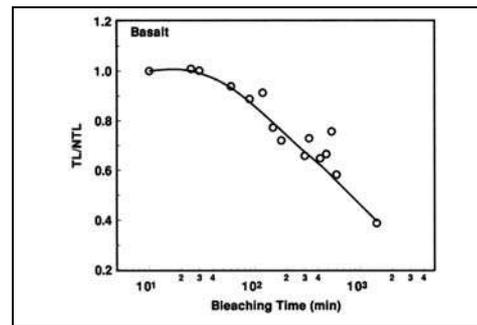
**Fig.15 EGBAS, basalt. Solar bleaching of TL as a function of bleaching time in a log scale.**
