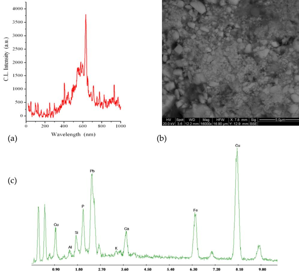
Fig. 5 a) CL spectrum was attributed to a copper and lead of matrix, b) SEM image of Cu-Pb matrix, c) EDX spectroscopy of Cu-Pb matrix
