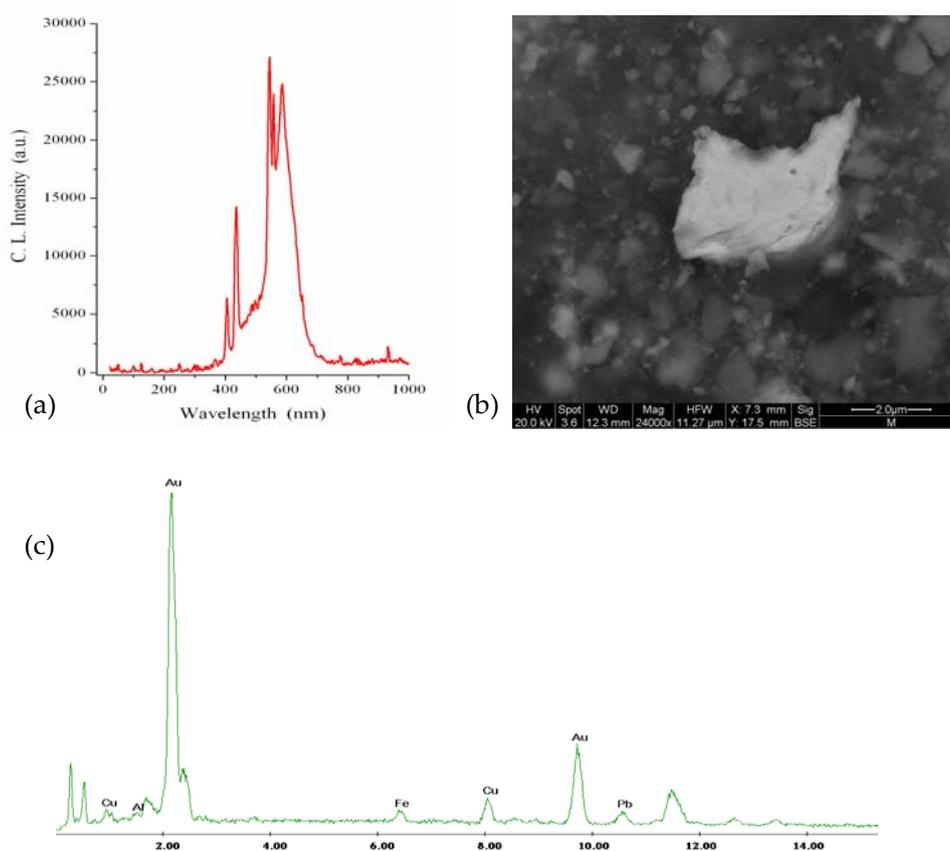
Fig 6 a) CL spectrum was attributed to gold particles, b) SEM image of Au particle, c) EDX spectroscopy of Au particle
