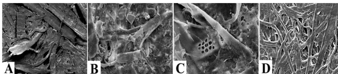
Fig. 6: Scanning electron micrographs of the untreated and aged untreated of the Rivista de Diritto Commerciale paper: (6A) Untreated sample (Magn. 600), (6B) Heat-moist-light aged untreated sample (Magn. 600), (6C) Heat-moist aged untreated sample (Magn. 600) (6D) Heat aged untreated sample (Magn. 600).
