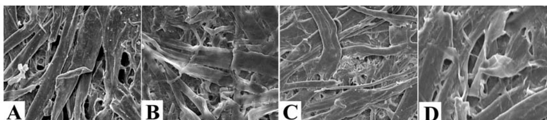
Fig. 5: Scanning electron micrographs of the treated and aged treated of the Austrian Book paper with chitosan at the second concentration: (5A) Treated sample (Magn. 900), (5B) Heat-moist-light aged treated sample (Magn. 1100), (5C) Heat-moist aged treated sample (Magn. 1000), (5D) Heat aged treated sample (Magn. 1000)
