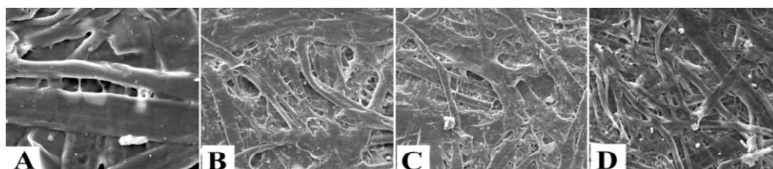
Fig. 7: Scanning electron micrographs of the treated and aged treated of the Rivista de Diritto Commerciale paper with cellulose acetate at the second concentration: (7A) Treated sample (Magn. 1100), (7B) Heat-moist-light aged treated sample (Magn. 1000), (7C) Heat-moist aged treated sample (Magn. 1000), (7D) Heat aged treated sample (Magn. 900)
