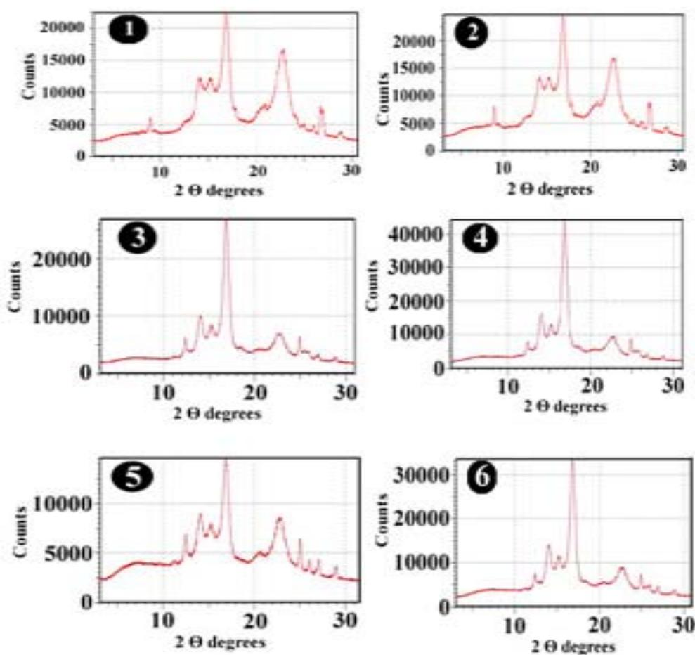
**Fig. 2: X-ray diffractogram of Rivista de Diritto Commerciale paper treated with cellulose acetate and chitosan at the second concentration before and after accelerated heat ageing cycle: (1) Untreated sample, (2) Heat aged untreated sample, (3) Treated sample with cellulose acetate, (4) Aged treated sample with cellulose acetate, (5) Treated sample with chitosan, (6) Aged treated sample with chitosan**
