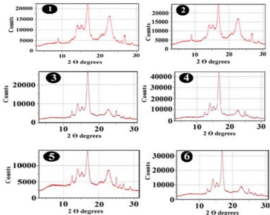
Fig. 1: X-ray diffractogram of Austrian Book paper treated with cellulose acetate and chitosan at the second concentration before and after accelerated heat ageing cycle: (1) Untreated sample, (2) Heat aged untreated sample, (3) Treated sample with cellulose acetate, (4) Aged treated sample with cellulose acetate, (5) Treated sample with chitosan, (6) Aged treated sample with chitosan
