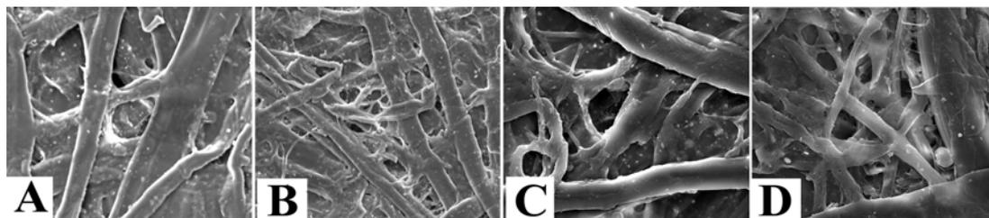
Fig. 4: Scanning electron micrographs of the treated and aged treated of the Austrian Book paper with cellulose acetate at the second concentration: (4A) Treated sample (Magn. 1300), (4B) Heat-moist-light aged treated sample (Magn. 1300), (4C) Heat-moist aged treated sample (Magn. 1300), (4D) Heat aged treated sample (Magn. 1300)
