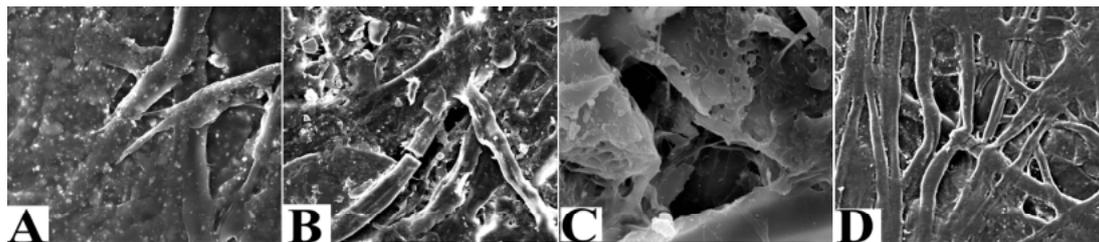
Fig. 8: Scanning electron micrographs of the treated and aged treated of the Rivista de Diritto Commerciale paper with cellulose acetate at the second concentration: (8A) Treated sample (Magn. 1000), (8B) Heat-moist-light aged treated sample (Magn. 1000), (8C) Heat-moist aged treated sample (Magn. 2000), (8D) Heat aged treated sample (Magn. 1000)
