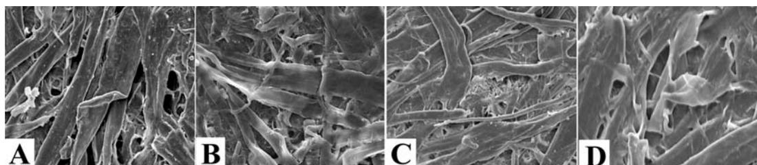
**Fig. 3:** Scanning electron micrographs of the untreated and aged untreated of the Austrian Book paper: (3A) Untreated sample (Magn. 1000), (3B) Heat-moist-light aged untreated sample (Magn. 1000), (3C) Heat-moist aged untreated sample (Magn. 1000) (3D) Heat aged untreated sample (Magn. 1000).
