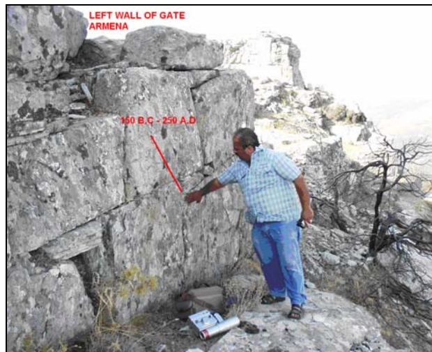
Fig. 5 Fortified wall at Armenia, left to the Gate entrance. Sampling and gamma reader.
