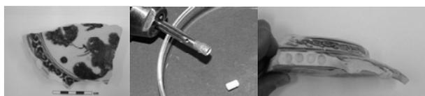
Figure 1. Drilling of core sample:  $d.= 3 \text{ mm}$ ,  $l.= 5 \text{ mm}$ .
