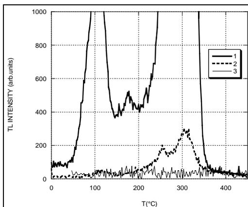
Fig. 4: Sample SL9: 1) glow curve obtained after 5 Gy beta irradiation 2) glow curve obtained after 5 Gy beta irradiation and 470 nm illumination for 20 s at RT 3) background emission.
