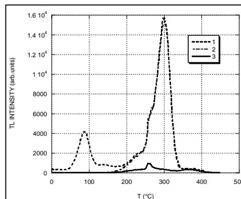
Fig. 2: Sample SL7. 1) glow curve obtained after a 5 Gy beta irradiation, 2) the same as in 1) with pre-heat at  $150^\circ\text{C}$  for 10s, 3) the same as in 2) with 470 nm illumination for 20 s at RT
