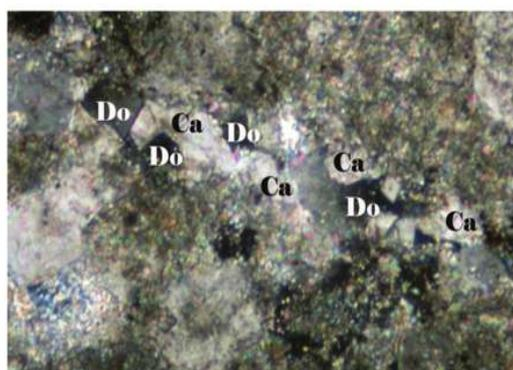
**Figure 7: Petrography of stone sample, calcite and dolomite crystals under polarized light, 500x**
