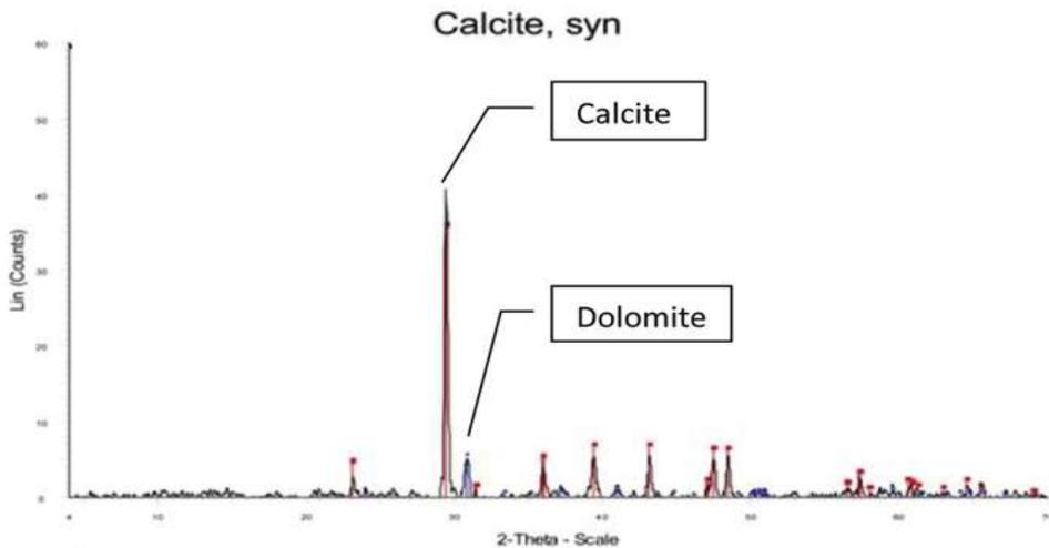
**Figure 9: XRD analysis of stone sample, red line indicates calcite and blue line indicates dolomite**
