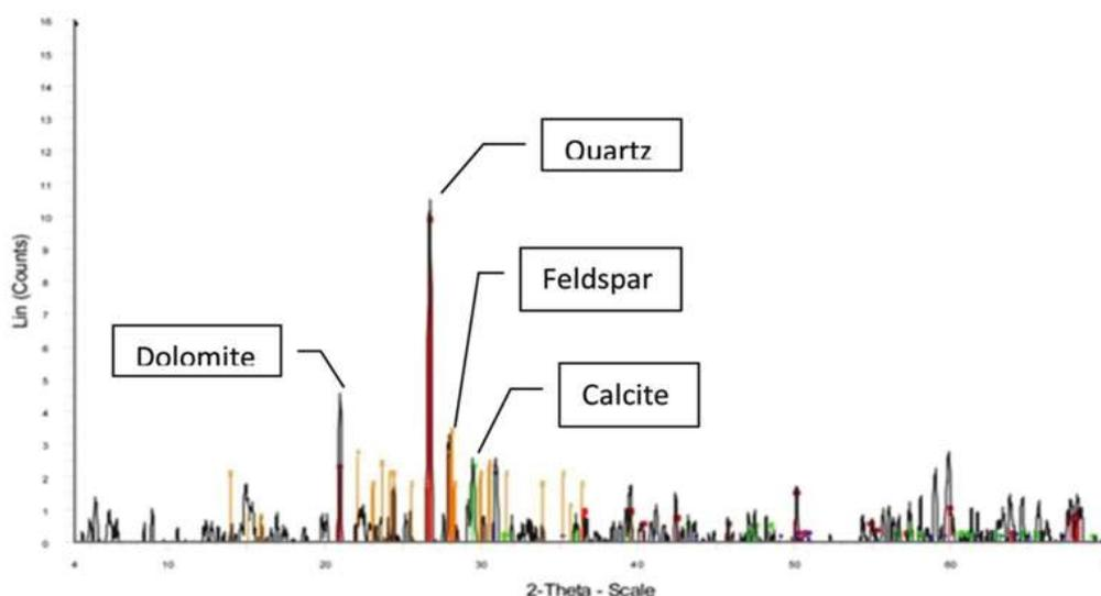
Figure 10: XRD analysis of sediments, indication of lines are as Red: Quartz, Blue: Dolomite, Green: Calcite and Yellow: Feldspar
