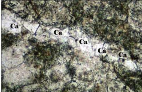
**Fig. 8: Calcite veins (white area) under normal light, 500x**
