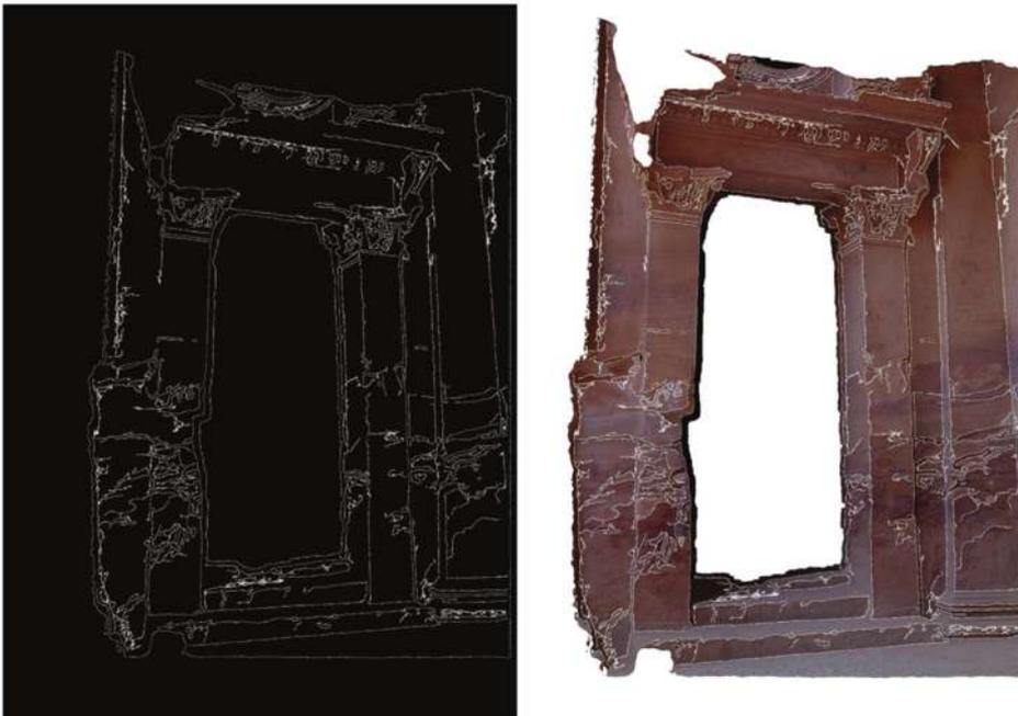
Figure 14. Image left, feature detection using canny operator convolved the true orthophoto. Image right, the segmentation results projected over the true orthophoto.
