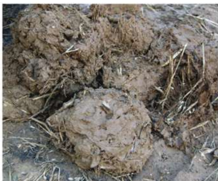
Figure 16: Balls of clay used for daubing of the walls. Sultana-Malu Roșu experiment.
