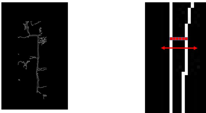
Figure 12. The binary edge map for the concern region using high threshold values, and measurement of the crack width
