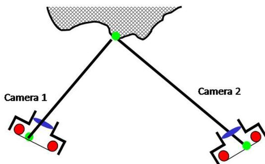
Figure 5. Principle of Photogrammetry for 3D Object Modelling
