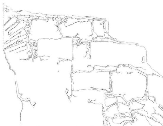
Figure 11. Binary edge map for the cracks extracted from true-ortho using canny operator.
