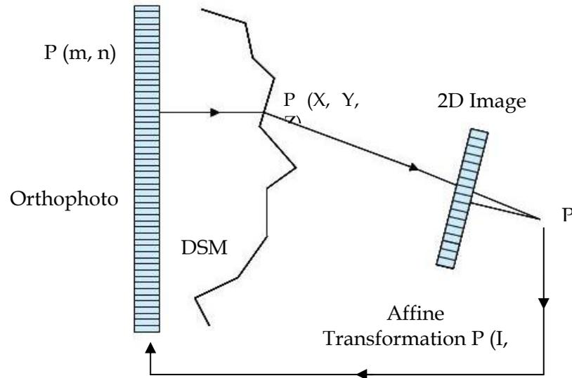
Figure 8. The true orthoimage framework production (After Alshawabkeh et al. 2010)
