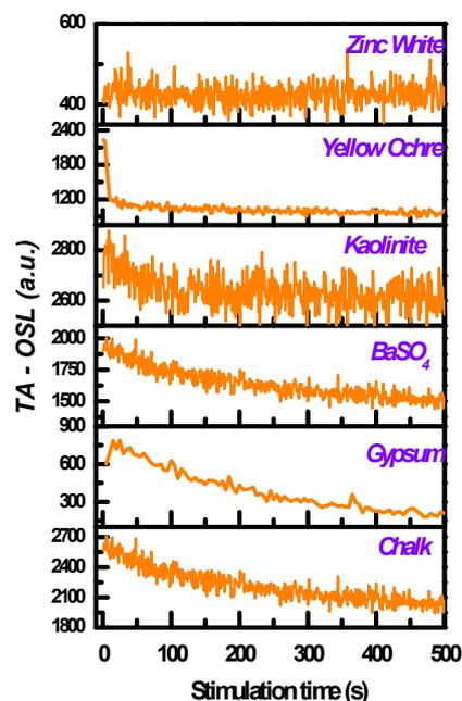
Figure 5. TA – OSL signal emanating from VDT for each material. Note the poor signal-to-noise ratio obtained for the case of zinc white, which is not indistinguishable from the background TA-OSL signal.
