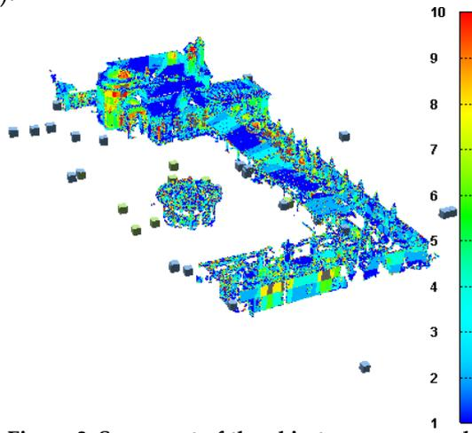
Figure 3. Some part of the objects were scanned many times with overlap measurements. The color legend on the right shows the repeated measurements (Red color shows 10 times measurement).
