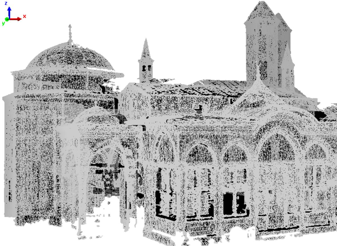
Figure 6 Triangulated point cloud model.
