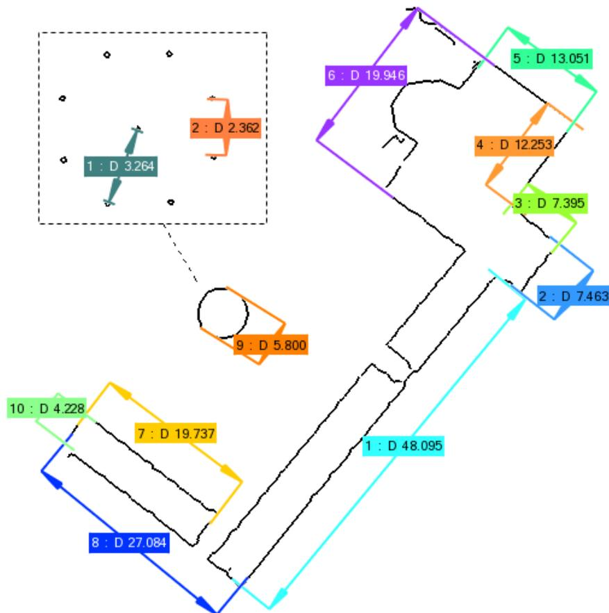
Figure 9 Ground plan that was created from cross-section of reference plane and point cloud and dimensions of the structures (units are meters).
