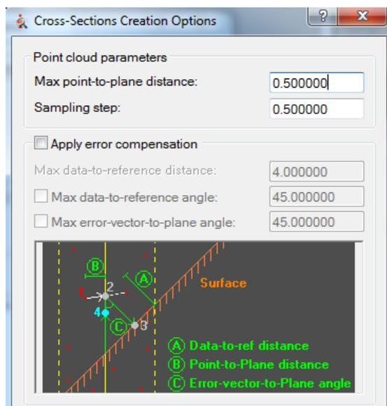
Figure 8 The cross-section parameters for creating ground plan (PolyWorks, 2007).
