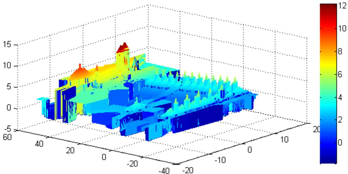
Figure 10 Digital elevation model generated from the point cloud data (units are meters).
