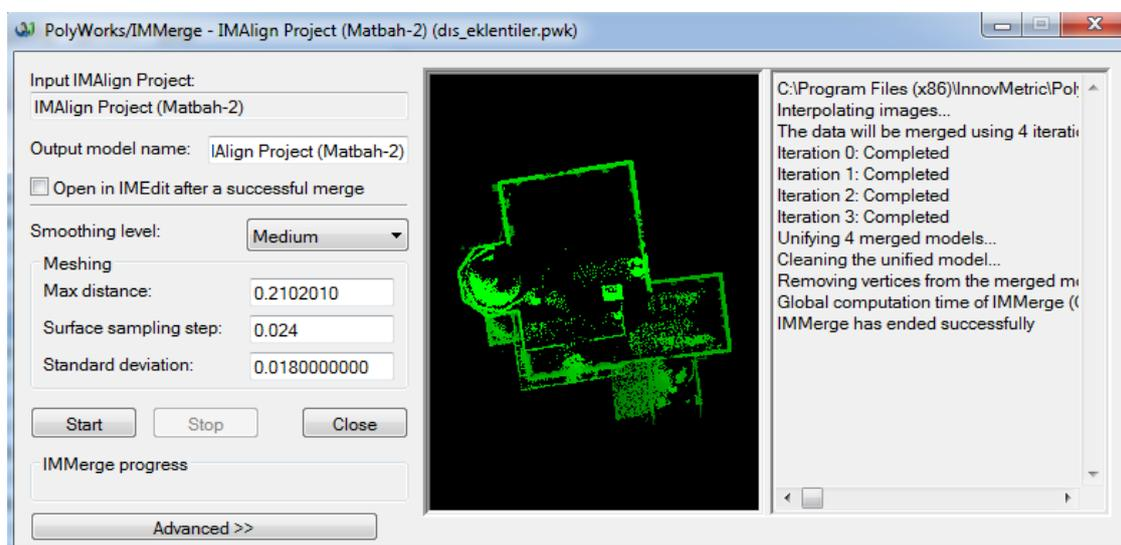
Figure 5. Setting and processing of the mesh creation from point cloud by PolyWorks.
