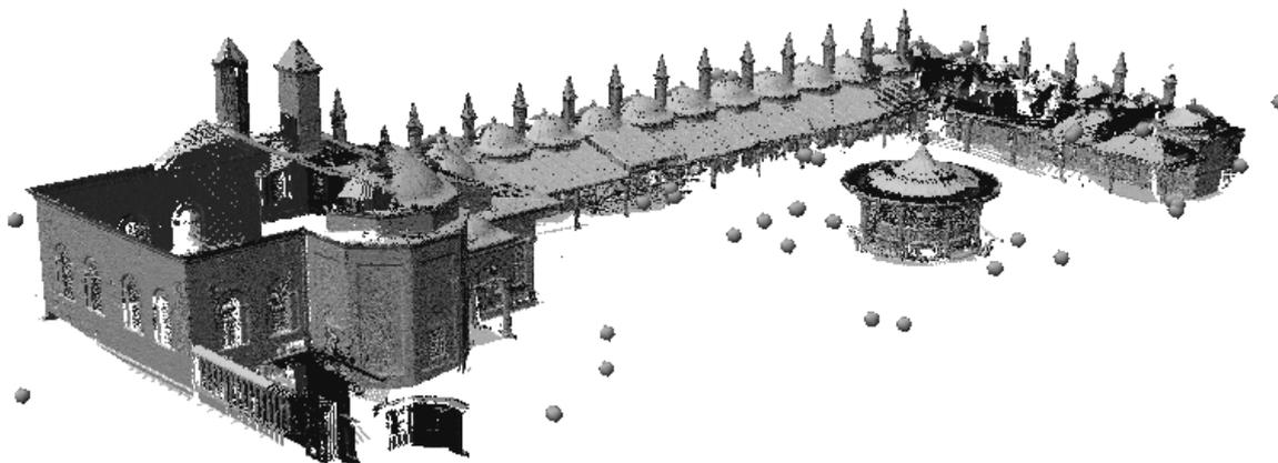
Figure 4. Generated point cloud model of the study objects. The points show the laser scanning stations.
