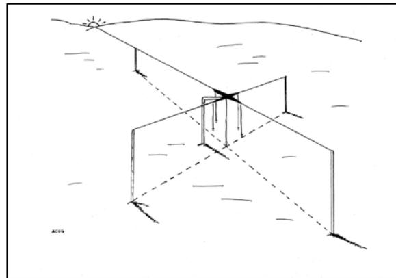
Figure 1: Possible reconstruction for the *groma* and its use to obtain the direction of the grid according to the path of the sun.
