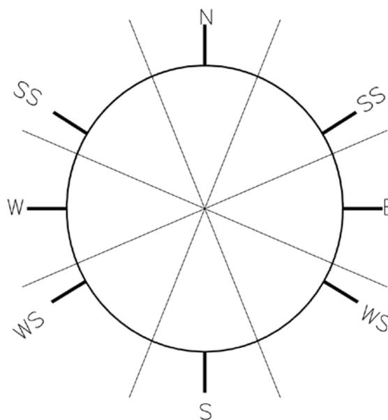
Figure 3: Diagram showing the eight divisions of the horizon used to obtain the main wind directions according to Vitruvius. The orientation of the city grid should avoid the central areas and thus follow the solid lines. Short heavy lines indicate the cardinal directions and the sunrise and sunset at the solstices (WS and SS).
