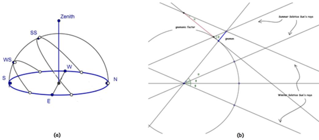
Figure I-1. Elements for the gnomonic factor (fg): (a) Sun's trajectories in a Horizon System at solstices (winter (WS) and summer (SS)); (b) Schematic view of the factor, including solstices' rays and shadows of a unitary gnomon;  $\theta$  is the Latitude of the site and  $\Delta$  represents the maximum solar declination (defining the Tropic of Cancer and Tropic of Capricorn); solar altitude above the Horizon is  $\alpha$  ( $\alpha$  for winter (summer) solstice).
