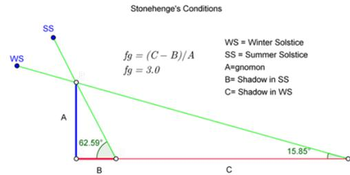
Figure 1 *Gnomonic factor (fg) definition. A gnomon defines two right triangles at different times, from its shadows and a light ray coming from the sun; both shadows are related with the extreme positions of the sun along the year (solstices). The numbers appearing correspond to the Stonehenge case.*
