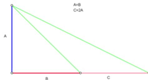
Figure 2. *Plato's Triangle definition. It is formed by two right triangles: one isosceles and other with sides  $1 : 2 : \sqrt{5}$ .*
