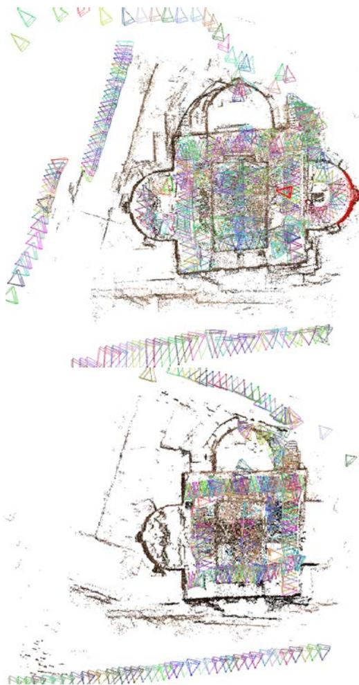
**Figure 7 Sparse Reconstruction and calibrated camera positions for Fountain of Peirene. User A (Top), and User B (Right), processed in VisualSfM.**
