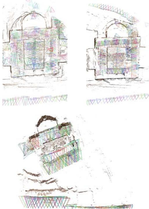
**Figure 9** Close-up of the sparse reconstructions and calibrated camera positions for Fountain of Peirene, User A (Top Left); User B (Top Right) (Processed in VisualSfM (Wu *et al.* 2011)).
