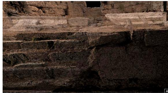
**Figure 4** A close-up of the steps and white marble in background shows that User B (Bottom) acquired a denser point cloud due to a higher megapixel camera and higher focal length.
