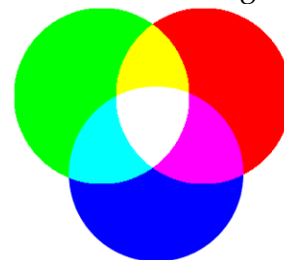
Figure 4: The production of white light by the mixing of the basic colors
