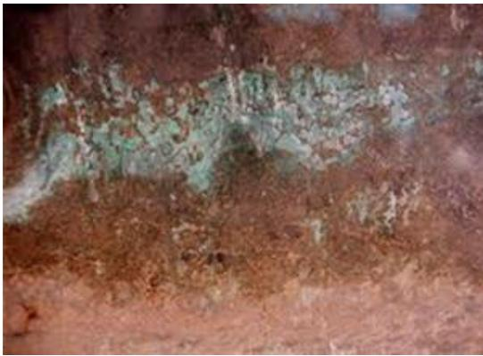
Figure 10. Microscopic image of strigil artifact shows the green color of malachite corrosion products.
