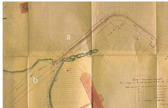
**Figure 3.** Project plan (1901) of the new L-shaped breakwater (a) built behind the ancient structure (b) (from State Archive of Lecce).
