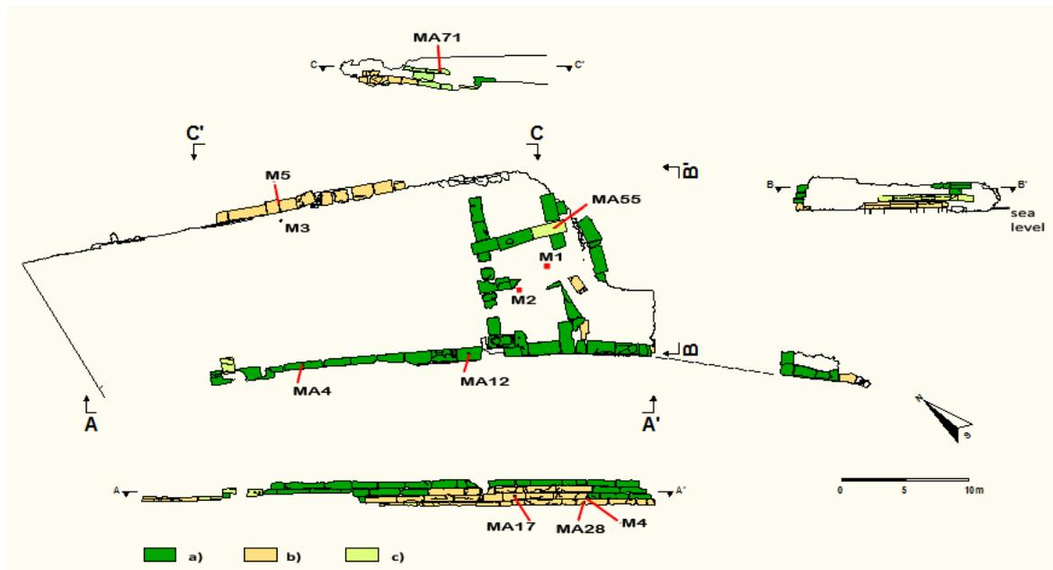
Figure 6 Distribution of the three varieties of miocene Pietra Leccese Fm. recognised in the roman pier: a) greenish limestone (Piromafo variety); b) straw yellow compact limestone, containing rare granules of glauconite; c) slightly glauconitic whitish-greenish limestone. In red, locations of collected samples.
