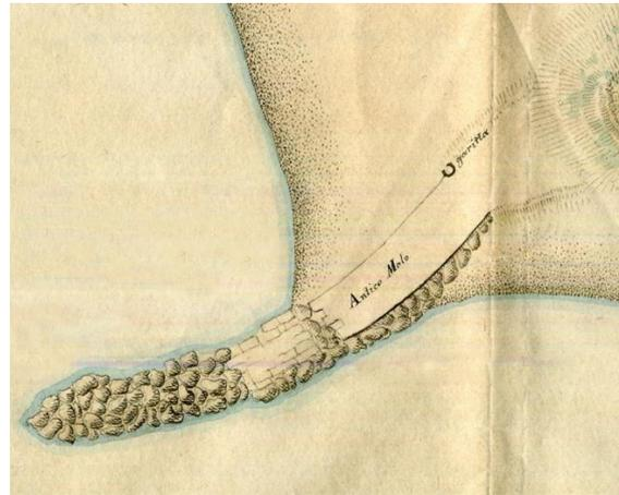
**Figure 2** Detail of historical map (1881) showing the original bending shape of the ancient pier (from State Archive of Lecce).
