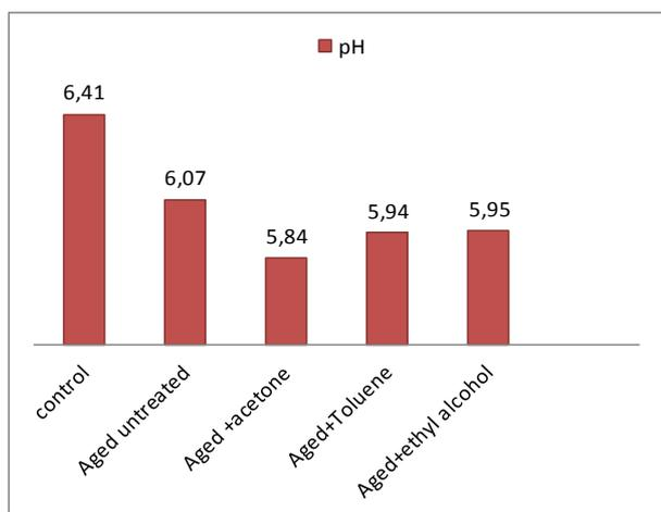
**Figure 2. pH values of untreated & treated paper samples after heat accelerated aging**
