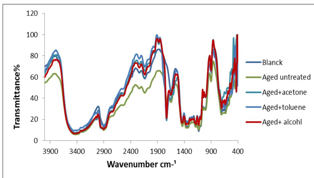
**Figure 2 . FTIR Spectra of paper samples before and after cleaning with acetone, toluene and ethyl alcohol upon heat accelerated aging**
