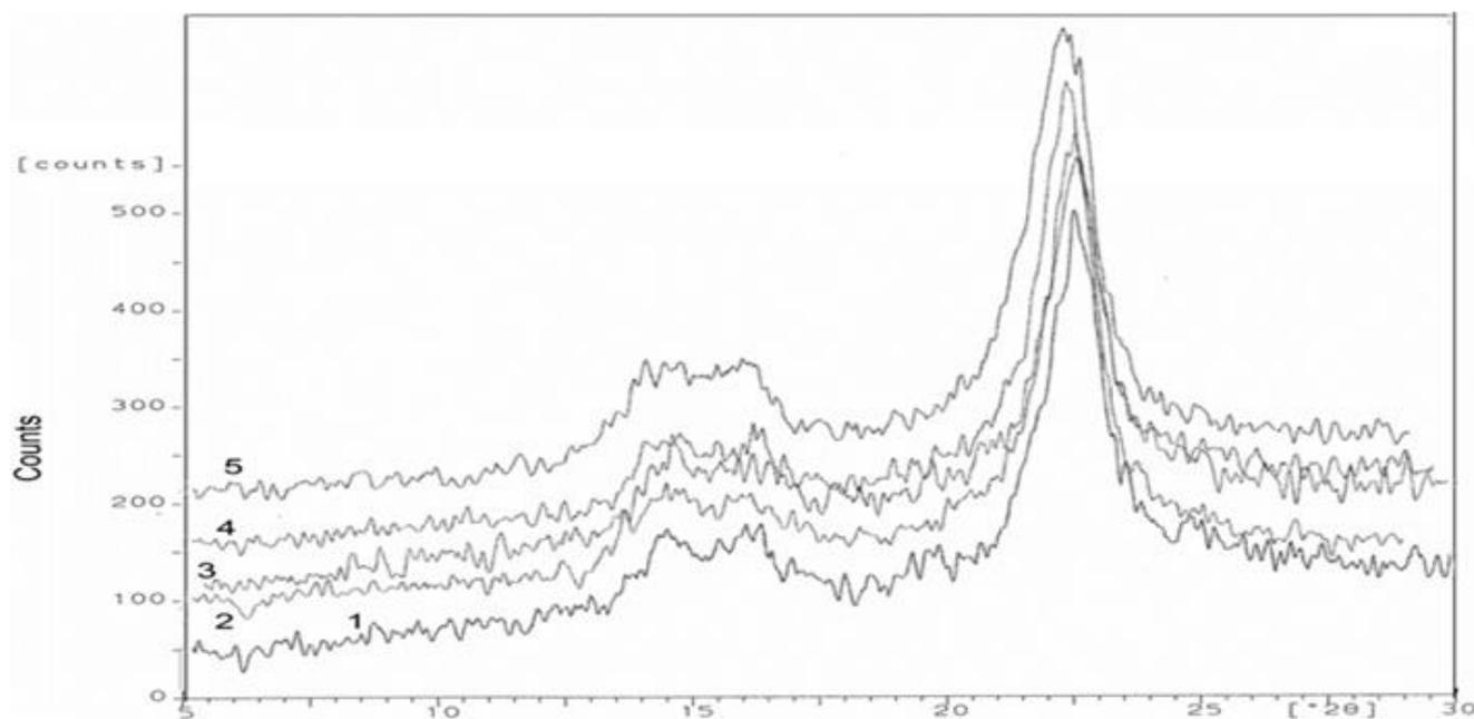
**Figure 3. X-diffactogram of samples of paper before and after heat aging (1) The control, (2) Aged untreated (3) Aged treated with acetone (4) Aged treated with toluene, (5) Aged treated with ethyl alcohol**
