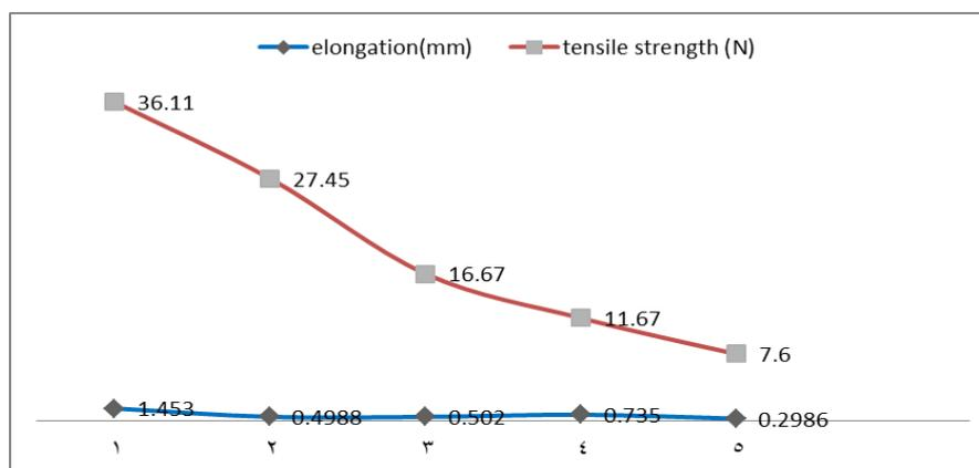
Fig . 1. Percent loss of tensile strength and elongation monitored for paper samples 1-5 exposed to heat accelerated aging
