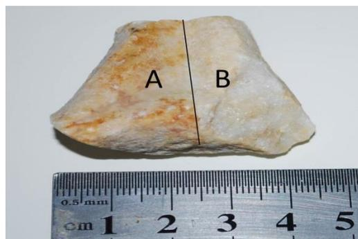
**Figure 8.** Iron rust stain on surface of marble artifacts on the left side (A), and the cleaned right side (B).
