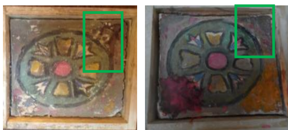
Figure 9 ( left ) The area of spot of wax in square area showing the area to be cleaned and (right) area cleaned by removing the wax spot using with magnetic nano gel using an external magnet.
