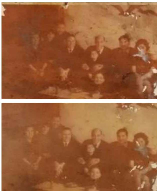
Figure 2. Sample 12 before (top) and after (bottom) cleaning with a 100% solution of toluene.
