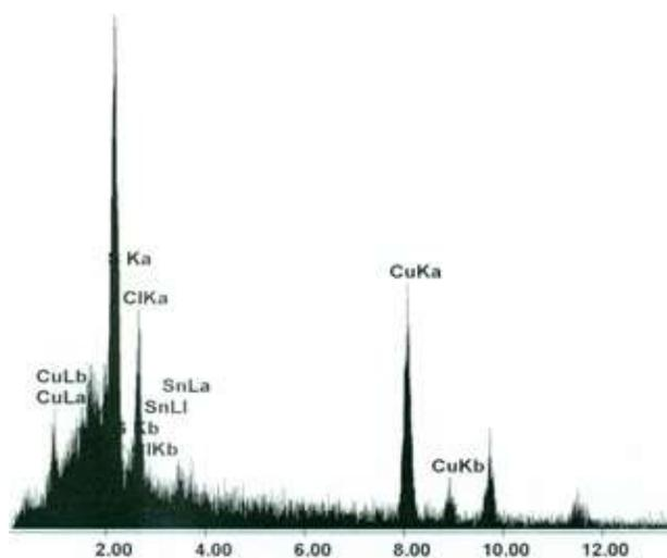
Figure 13. EDX analysis of the blank sample versus the 0.5M sodium chloride corrosive solution
