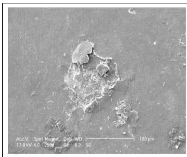
Figure 14. SEM analysis of the coupon surface containing inhibitor in the presence of 0.5M sodium chloride corrosive solution
