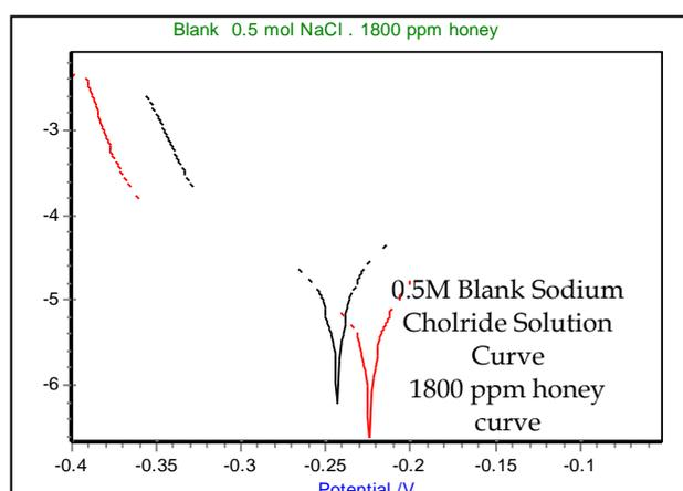
Figure 3. Polarization curve pertaining to honey in 1800 ppm concentration
