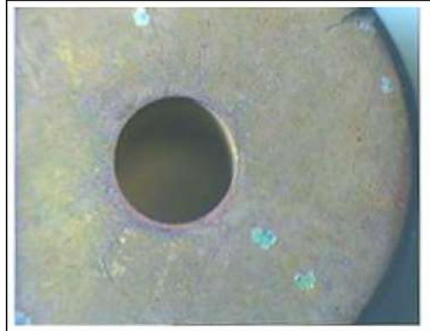
**Figure 11.** Corrosion of the coupon surface in a 1200 ppm honey concentration, magnified 40X
