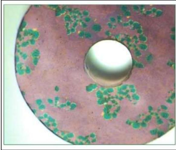
**Figure 8.** Coupon in corrosive solution of 0.5M sodium chloride after 30 days of floatation, magnified 40X
