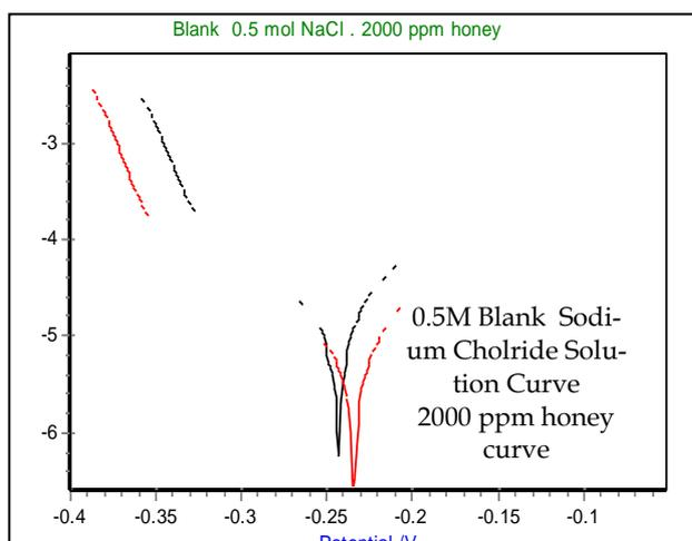
Figure 4. Polarization curve pertaining to honey in 2000 ppm concentration
