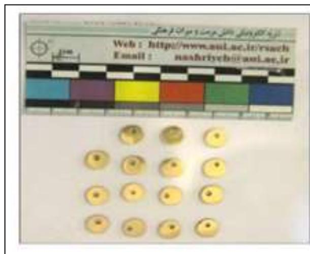
Figure 6. coupons prepared for soaking
