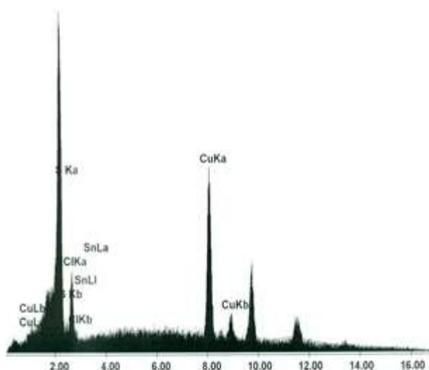
Figure 15. EDX analysis of the coupon surface containing inhibitor in the presence of sodium chloride corrosive solution
