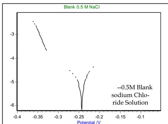
Figure 1. Tafel polarization curve for 0.5M sodium chloride
