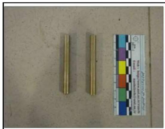
Figure 5 Electrodes prepared for the coupons' incision.
