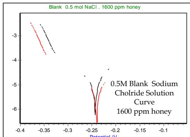
Figure 2. Polarization curve pertaining to honey in 1600 ppm concentration
