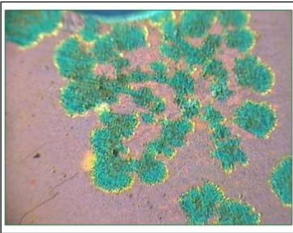
**Figure 9.** Coupon in 0.5M sodium chloride corrosive solution after 30 days of floatation, magnified 60X
