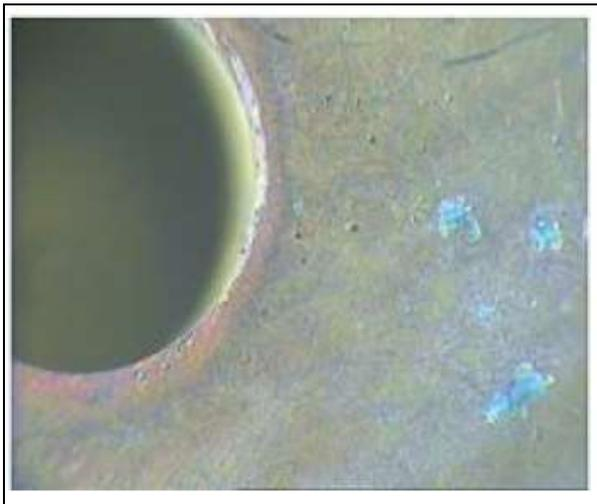
**Figure 10.** Corrosion of the coupon surface in 1200 ppm concentration of honey, magnified 80X
