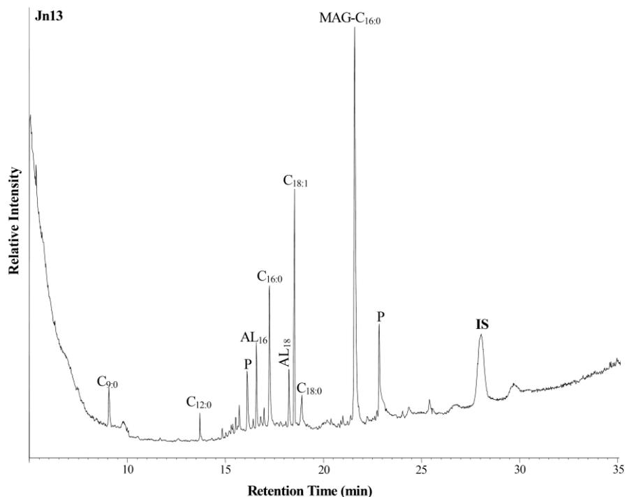
Figure 2. Partial (0-35 min) total-ion-chromatogram (TIC) of the trimethylsilylated total lipid extract of the organic residue obtained via conventional solvent extraction from the interior of sherd Jn13. ( $C_{x:y}$ ): monocarboxylic fatty acid of carbon chain length  $x$  and degree of unsaturation  $y$ , (MAG- $C_{x:y}$ ): monoacylglycerol with  $C_{x:y}$  fatty acid moiety, (P): plasticizer, and (IS): the internal standard (*n*-tetratriacontane;  $C_{34}$ ).
