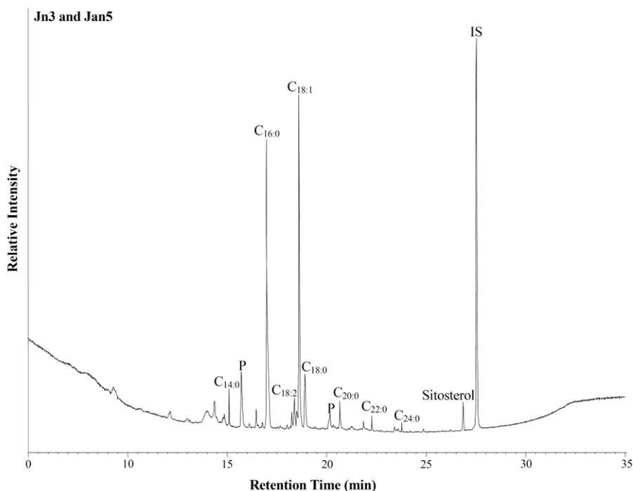
**Figure 1. Partial (0-35 min) total-ion-chromatogram (TIC) of the trimethylsilylated total lipid extract of the organic residue obtained via conventional solvent extraction from the interiors of sherds Jn3 and Jn5. (C<sub>x:y</sub>): monocarboxylic fatty acid of carbon chain length x and degree of unsaturation y, (P): plasticizer and (IS): the internal standard (*n*-tetratriacontane; C<sub>34</sub>).**
