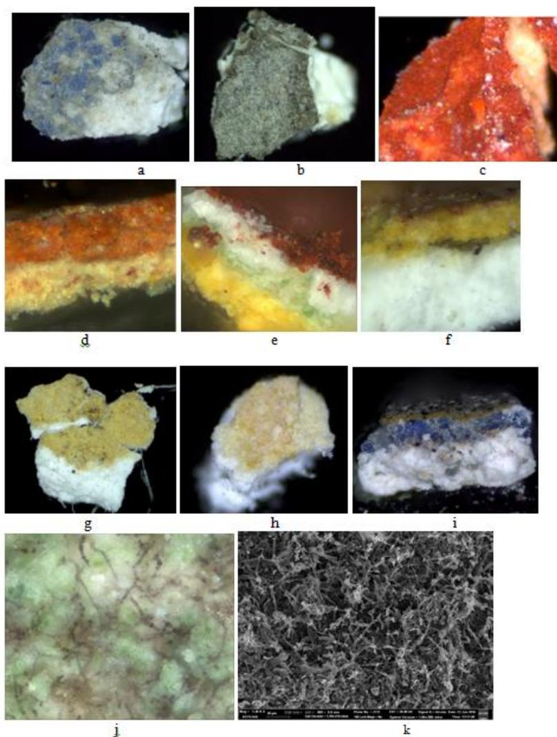
**Figure 5.** OM images: a - blue background (after the restoration), b - grey background (before the restoration), c - red paint of the fresco framing, d - red paint of the cloak, e - brown paint of the armour contour, f - orange paint of armor, g, h - yellow paint of the armour and background, i - dark-beige paint of the horse head green paint of the; j, k - OM and SEM image of the green (sleeves) region.
