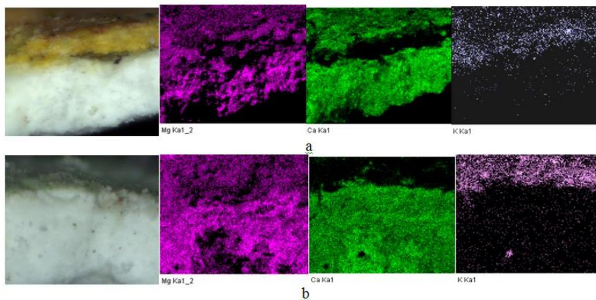
Figure 3. Mapping of Mg, Ca and K distribution for the sample; a) represents the orange pain of the armour, b) represents the green paint of the sleeve.
