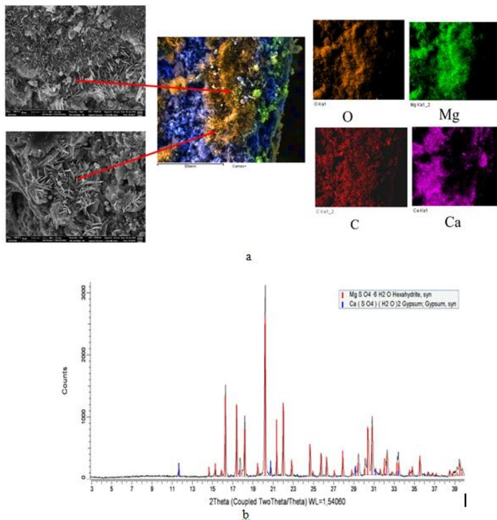
Figure 4. a - SEM- images and cartograms of O, Mg, C and Ca distributions; b - X-ray pattern of the white fluffy coating from the moisturized wall.
