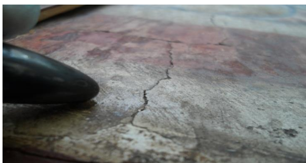
Figure 3: The magnetic nano materials don't affect by the external magnet as it penetrates the porous of the mural painting being connected with it's structure.
