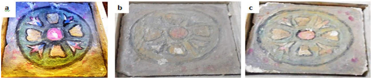
Figure 5: (a) the model before the treatment of magnetic nano- materials, (b) and (c) the model after the treatment of magnetic nano materials.
