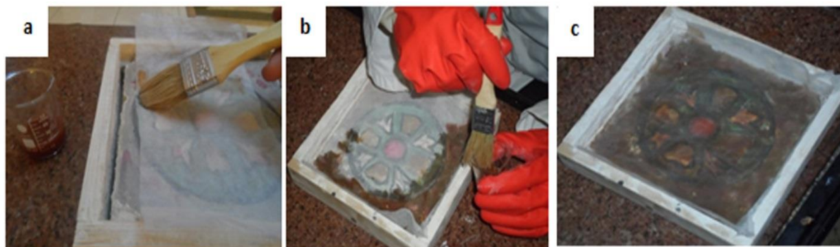
Figure 2: (a, b) The application of the suspension of nano-magnetic material using brush through Japanese paper, (c) The appearance after application
