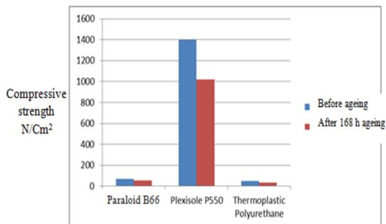
Fig. 12 Effect of artificial ageing on Compressive strength of the three polymers.
