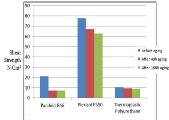
Fig. 10 Effect of artificial ageing on shear strength of the three polymers.
