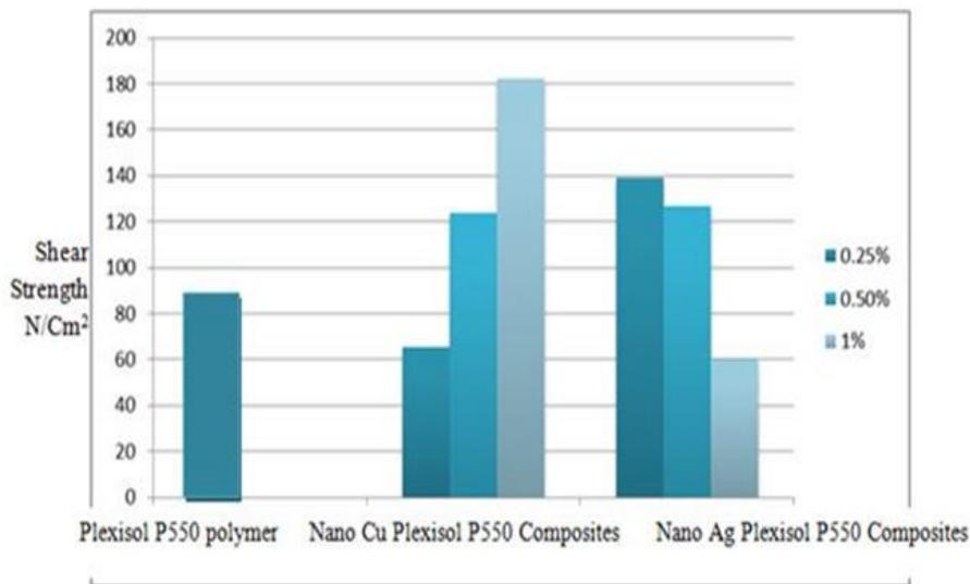
Fig. 13 Shear Strength results of Plexisol P-550 Polymer , Nano Copper & Nano Silver Plexisol P-550 Composites.
