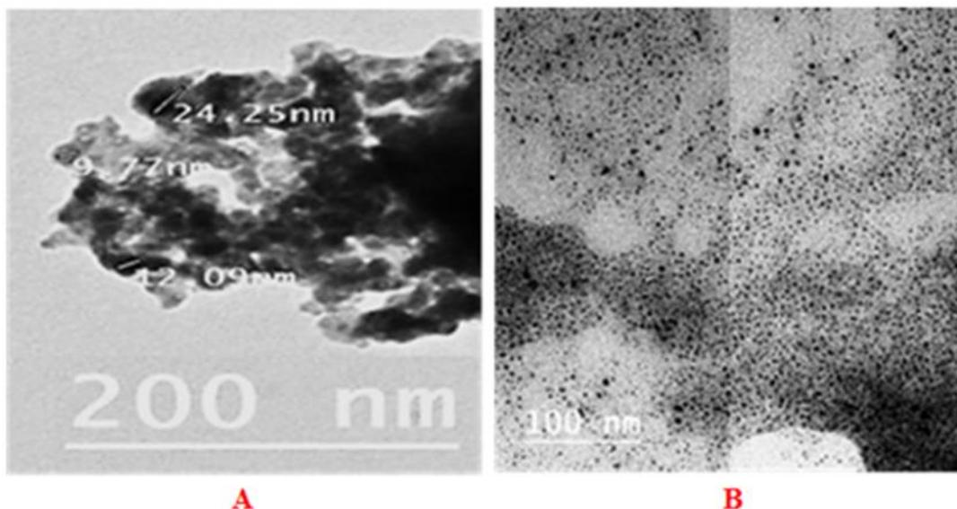
Fig. 2. TEM images of nanoparticles. (A) Nano copper (200 nm scale), (B) Nano silver (100 nm scale)
