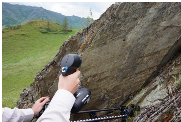
Figure 5. 3D scanning of the surface for deviation control of the final model.
