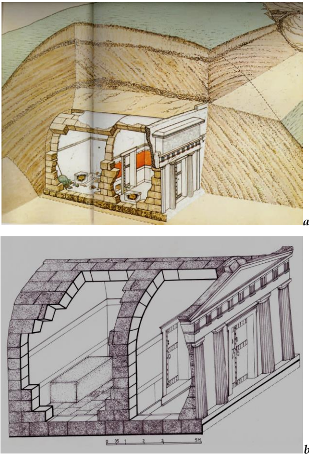
Figure 1. a) 3D reconstruction drawing of Philip II tomb from the Great tumulus at Vergina (after Andronikos 1989, 99). Behind the Doric façade we can see the antechamber and the main chamber, the marble door connecting them, the barrel-vault and the tumulus. b) Axonometric reconstruction of the Macedonian tomb D at Pella. (Haddad, 1999, 165).
