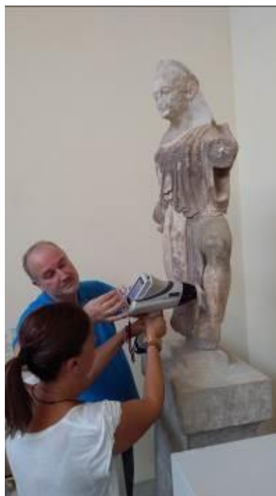
Figure 2. XRF measurement on a Marble cape from the archaic temple of Apollo (Artefact's numbering in Museum's catalogue: 4815), see Table 1.
