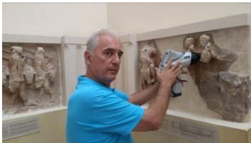
Figure 1. XRF measurement on an Embossed forked metopes of the Sikyonian treasure (hall III) (Artefact's numbering in Museum's catalogue: 1323, 1210 & 1381) see Table 1.
