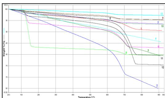
**Figure 3.** Thermogravimetric analysis (TGA) of ceramic samples (Numbers 1-13 in graphs represents the samples from BH-B1 to BH-B13).
