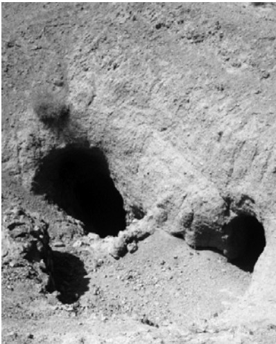
Figure 4b. The tunnels dug parallel to the ore body
