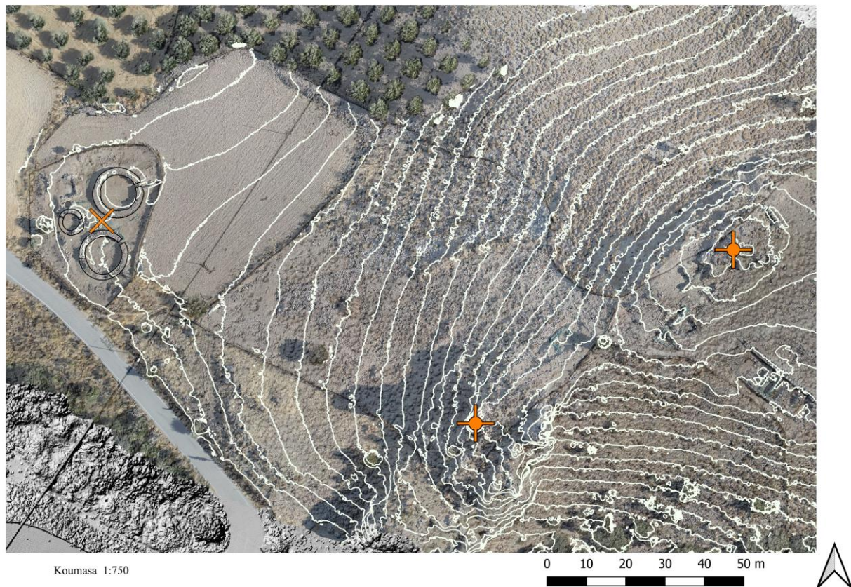
Figure 2. Orthophoto of the Koumasa slope, with 2m isometric lines. The two peaks are marked with a cross and the 'x' between the tholoi marks the observation point for measurements and from which the panorama of Figure 3 was observed. 10
