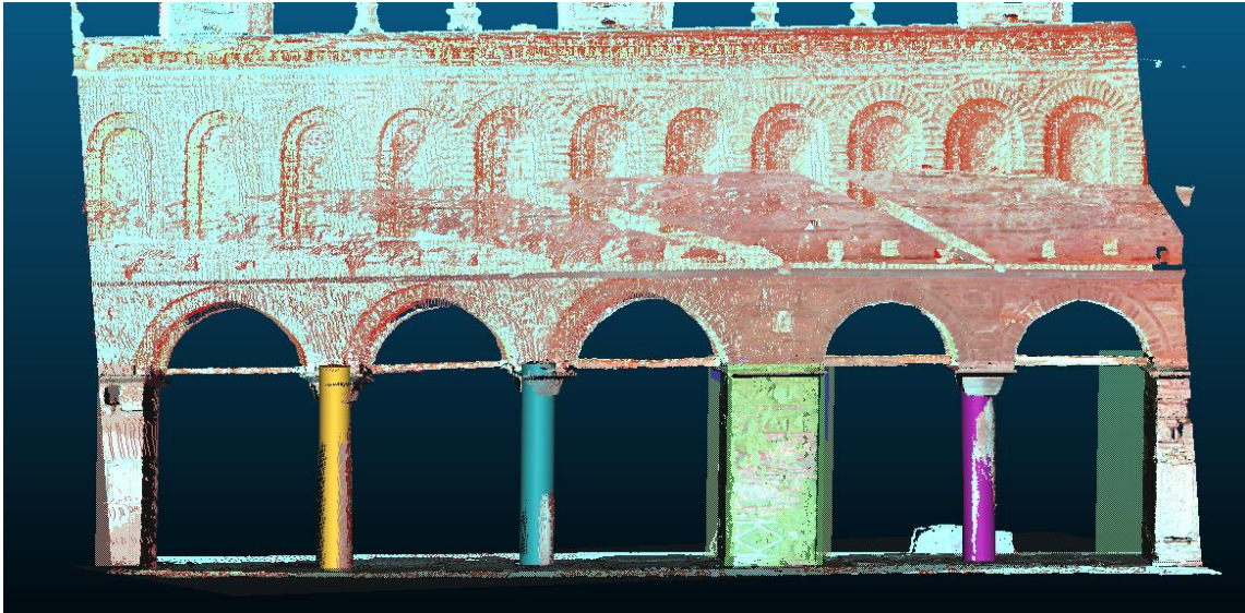
Figure 4. CloudCompare HBIM Models for Columns with RANSAC Algorithm
