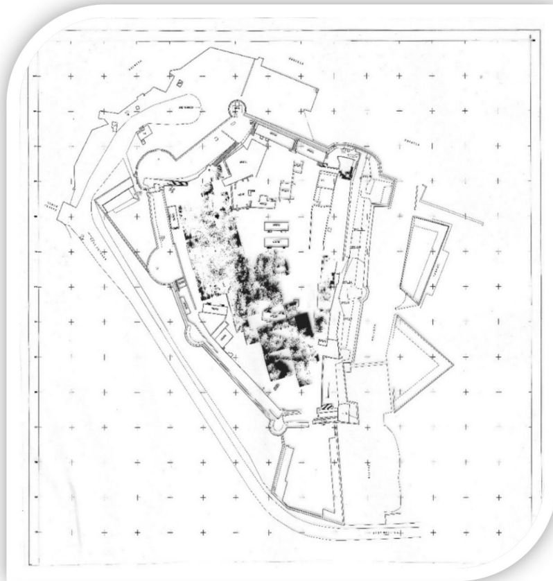
Figure 4. First Presentation of the Results. Image of the Resistivity Distribution in the Fortress of Lefkas (Liritzis et al., 1997)
