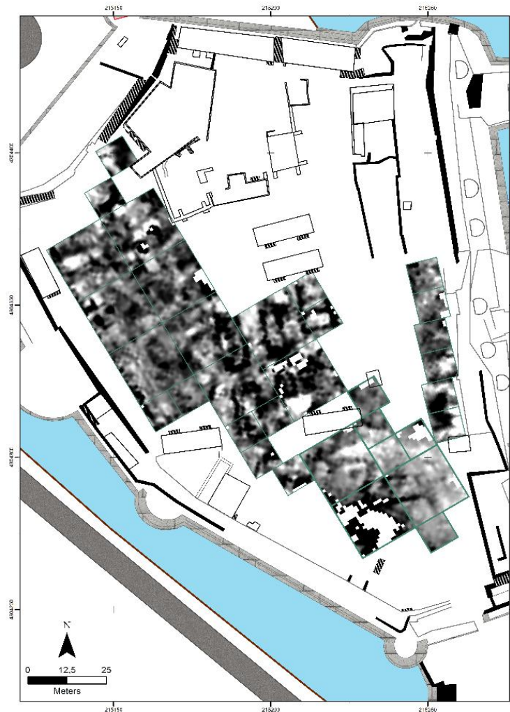
Figure 5. Resistance Distribution in the Fortress of Aghia Maura in Grey Scale Mode. Dark Tones Represent High Resistances
