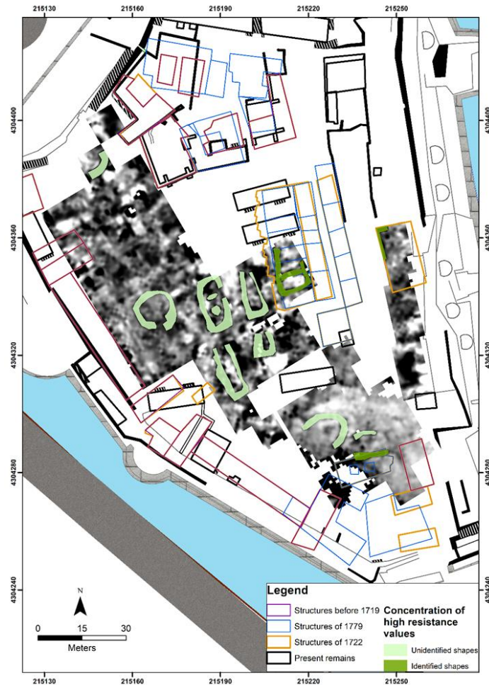
Figure 11. ER Results Combined with Features of All Phases. Unidentified Shapes are Emphasized
