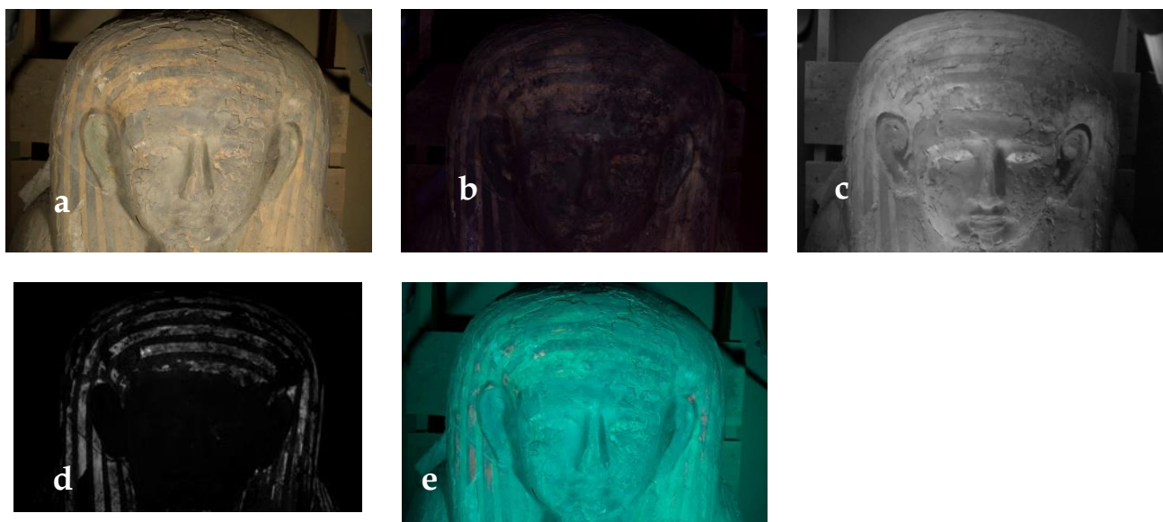
Figure 4. Technical images for the face area of the coffin made by different methods a) visible (VIS), b) Ultraviolet Fluorescence (UVF), c) infrared (IR), d) Infrared fluorescence (IRF), e) infrared false color (IRFC).
