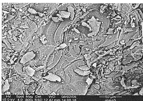
Fig. 6: Backscattered electron image of sample G. 1 showing the fractures and dissolution voids of devitrified area of corroded surface.
