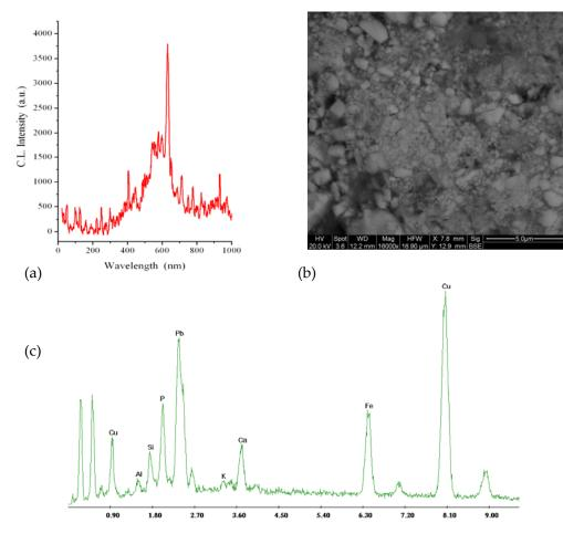
Fig. 5 a) CL spectrum was attributed to a copper and lead of matrix, b) SEM image of Cu-Pb matrix, c) EDX spectroscopy of Cu-Pb matrix
