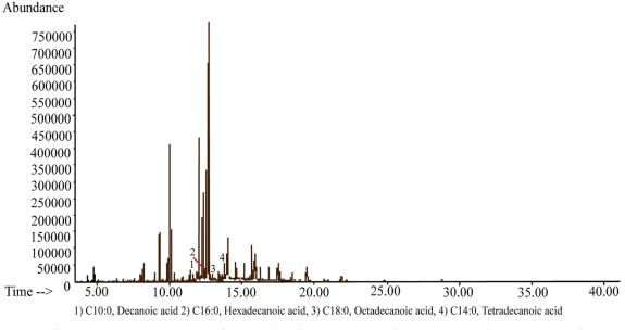
Figure 5: Chromatogram of Base Ring juglet 6062.16 (second analytical parameter)
