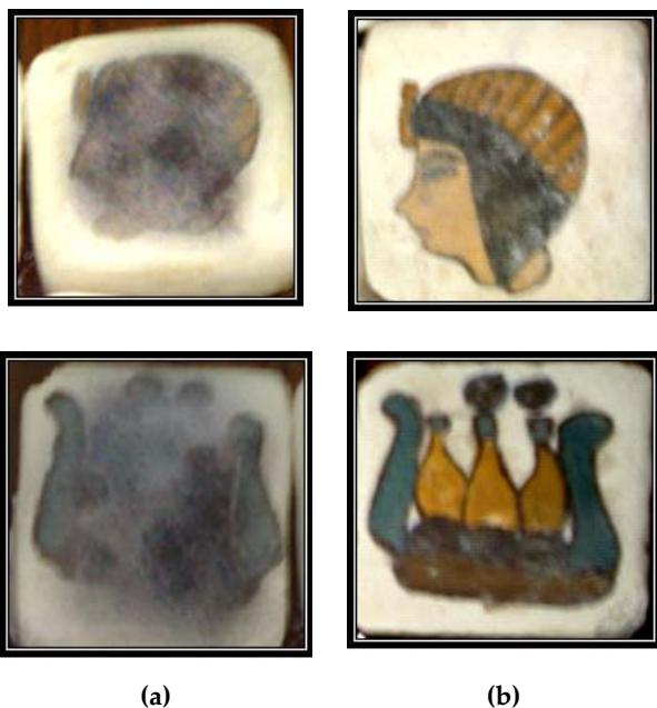
Fig. (7) Deteriorated mural models by Aspergillus niger (a) before treatments (b) after treatment and leaving for 30 days
