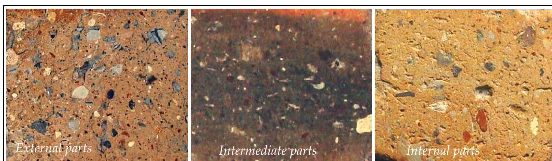
Fig. 6: Different colors and texture features of brick samples
