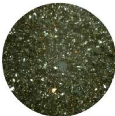
Figure 29. Sample No. 4 Tape Kelar. XPL Light, silty texture, large number of quartz in light color
