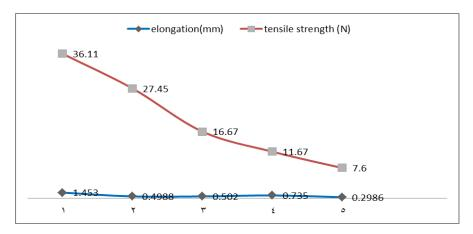
Fig . 1. Percent loss of tensile strength and elongation monitored for paper samples 1–5 exposed to heat accelerated aging
