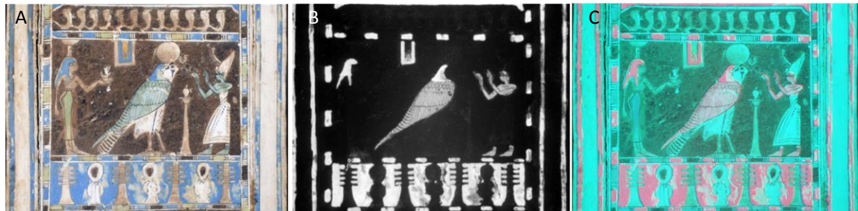
Figure 15. Technical photography of Egyptian Blue pigment A. Visible light (VIS) B. Visible induced Infrared luminescence (VIL) C. Infrared false color (IRFC)
