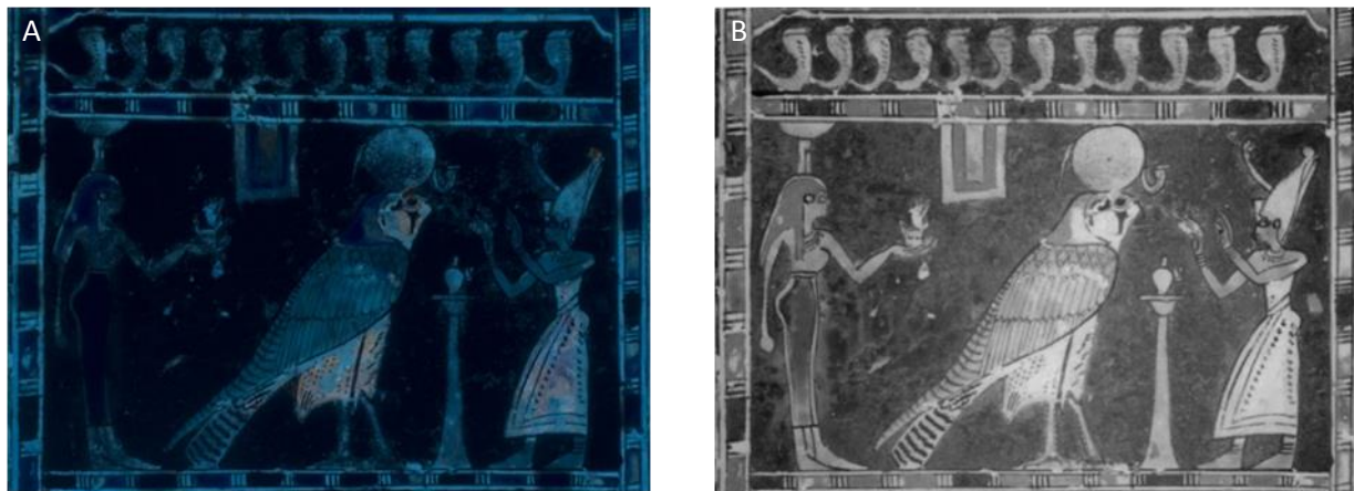
Figure 26. Technical photography of painting medium: (A) The ultraviolet-induced luminescence (UVL) image; black pigment appear darker, (B) IR image; hidden black outlines below the sand and dust layers appeared, and carbon black color is sharp.
