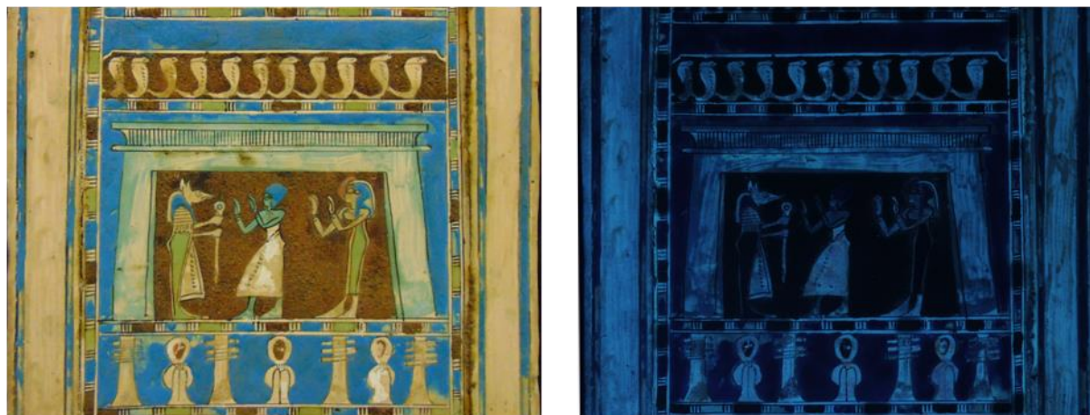
Figure 23. Technical photography of painting medium: (A) visible light. (VIS) (B) The ultraviolet-induced luminescence (UVL) image showed evidence for the presence of adhesive or organic material as splashes by brushes.
