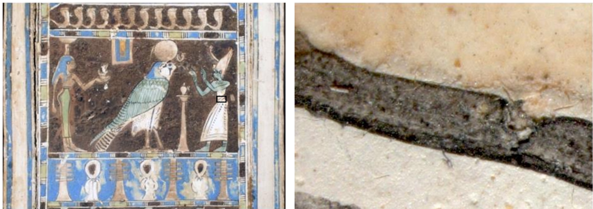
Figure 25. Black pigment under microscope showed homogeneous distribution of a fine-grained black.
