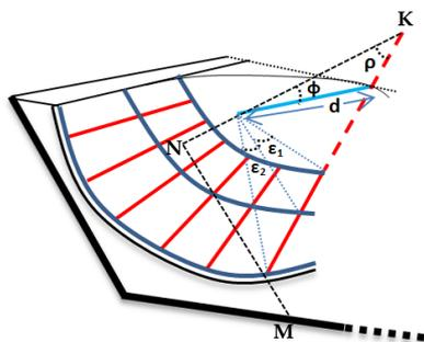
Figure 2. Schematic presentation of a conical sundial. In the figure, the angle ( $\rho$ ) formed between the cone-axis (dark dashed line) and the generatrix (red dashed line), the geographical latitude ( $\phi$ ) of operation, the length ( $d$ ) of the gnomon (bold blue line) and the angles of the obliquity of the ecliptic ( $\epsilon_1=\epsilon_2=\epsilon$ ) are marked.
