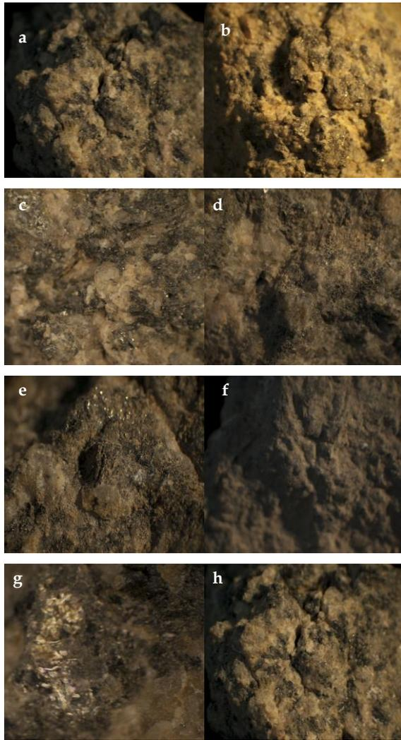
Figure 10 micrographs of investigated samples by LOM (4X) Granular disintegration, fractured, cracks, Exfoliation, cracks, voids, concentrated layer of dirt and mica noticed clearly.
