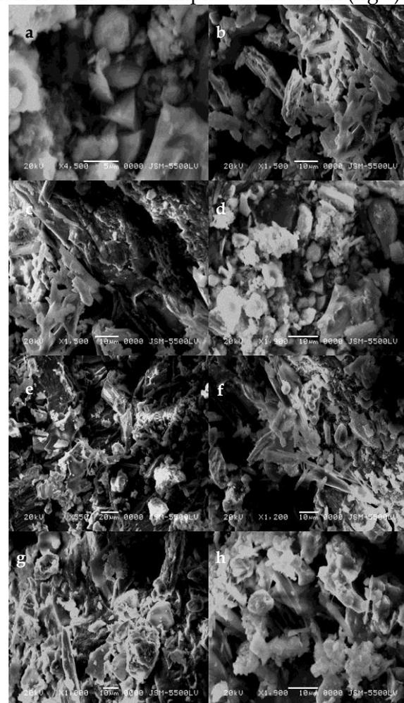
**Figure 8** SEM photomicrographs of the diorite samples a,b- deformation of internal structure of diorite; c- micro exfoliation and pitting; d- disintegration; e,f- sodium chloride crystals; g,h- crystal of gypsum.
