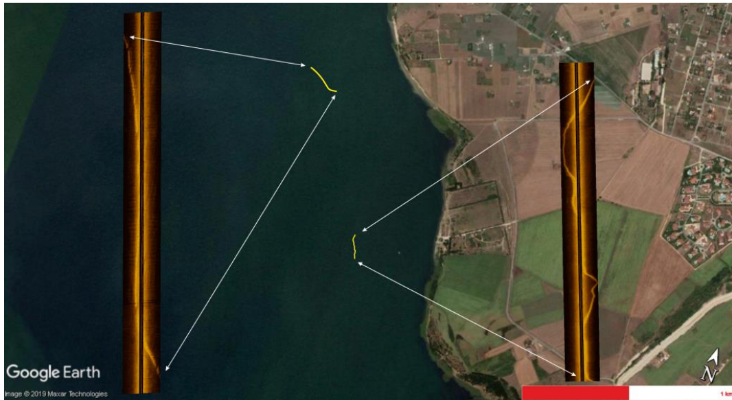
Figure 8c. Detected embankment lines to show possible continuity - photomosaics of the sonar images of the embankment.
