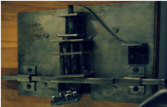
Figure 12 a) Roman smart Laconian from Jerash in Jordan. b) Haddad axonometric reconstruction of the smart Laconian Lock (After Haddad, 1995, plate 114). c) Recent reconstruction model of smart Laconian Lock smart Laconian Lock, (After https://museumsaskew.files.wordpress.com/2013/08/lock5.jpg ).
